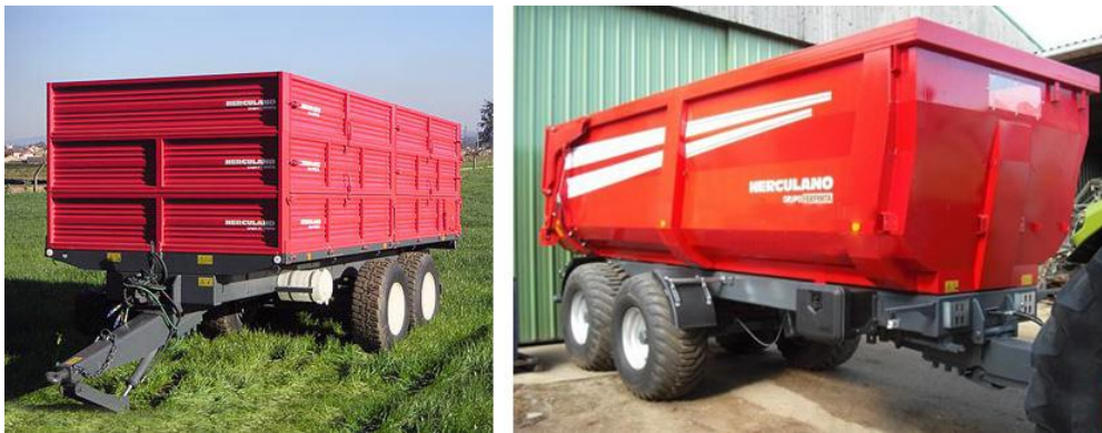
Figura 87. Reboques Herculano: Taipal 16 t / 21.6 m 3 (esq.); Monocoque 16t / 18 m 3 CCU
