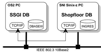
*Figure 4 - Shop-floor Database Replication Application*
