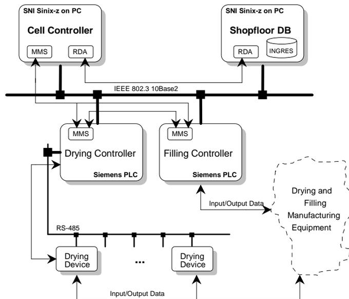
**Figure 2 - Drying and Filling Application**
