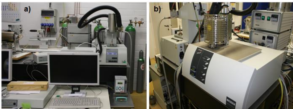
Figure 12: a) Simultaneous TG-DTA/DSC-Apparatus; b) Mass spectrometry MS403C.
