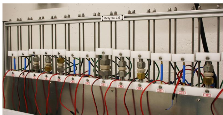
Figure 11: Batteries testing in BaSyTec equipment.
