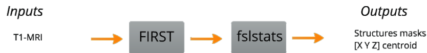
Figure A.5: Workflow applied for the segmentation of DBs and the estimation of their centroid, using FSL.
