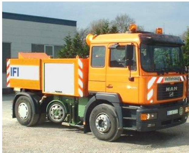
Figura 27 – SCRIM (Sideways Force Coefficient Routine Investigation Machine) [SCRIM Messungen. Disponível em: http://www.ifi.de/scrim.htm ]
