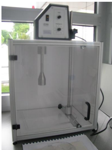
Figure 10: Ultra sound mixer with ultrasonic probe (UP200s) from the company Hielscher- ultrasound technology
