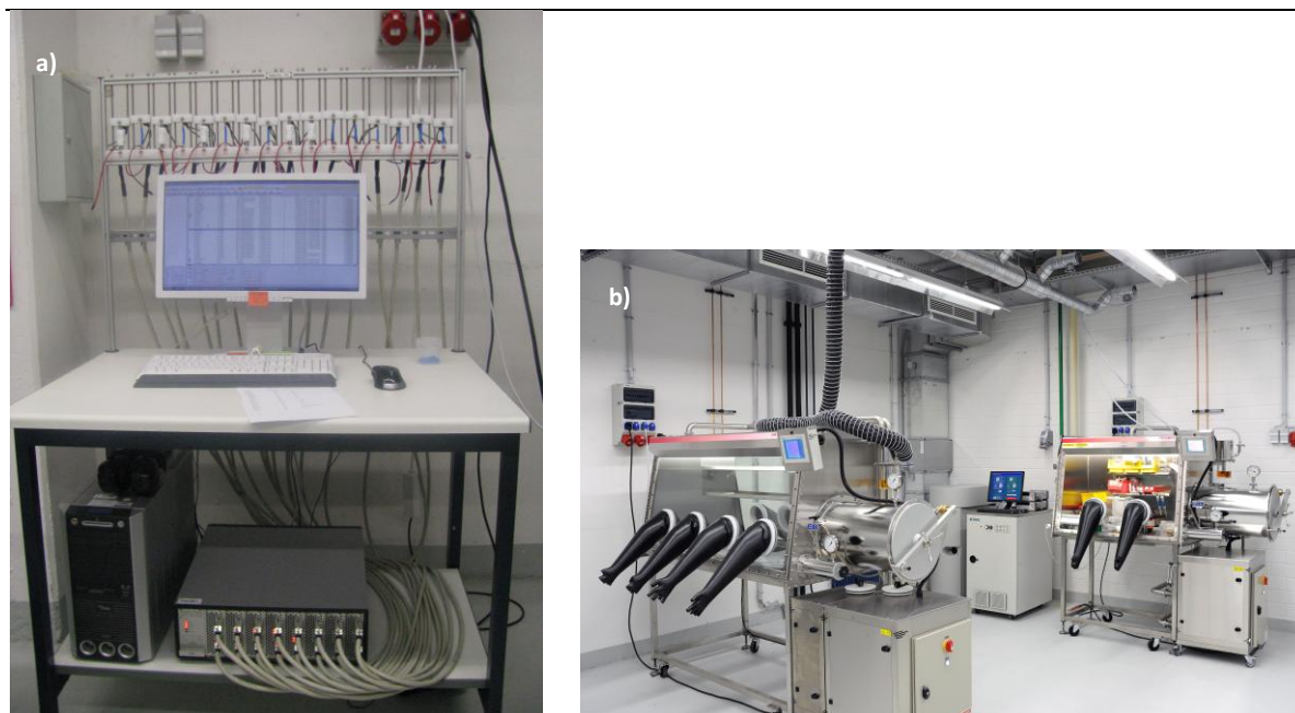
Figure 13: a) BaSyTec test equipment, with 16 channels to test batteries simultaneously. The batteries are testing in the top; b) Glove boxes used for the preparation of batteries.
