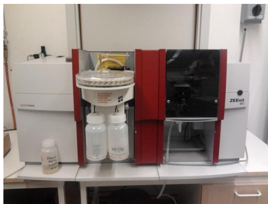
Figure 7 Atomic absorption spectrophotometer used for analyses.
