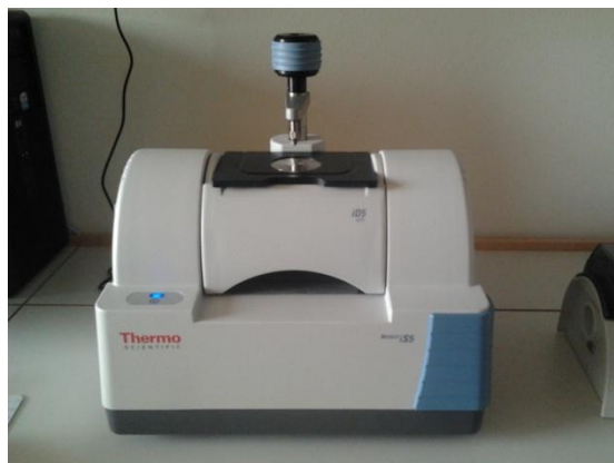
Figure 5 FTIR spectroscope used for analyses.
