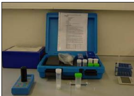
Figura 8. Componentes do kit RemediAid - Total Petroleum Hydrocarbon Test Kit (da AZUR Environmental).
