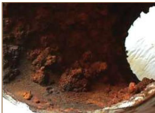
**Figure 1-** Ductile iron pipe section from DWDS with a biofilm and high amounts of corrosion products (Chaves Simões and Simões 2013).
