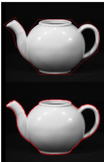
Figure 5: Initial contour (top); result of the segmentation process using r=2,000\text{N/m} and considering a rubber model (bottom).
