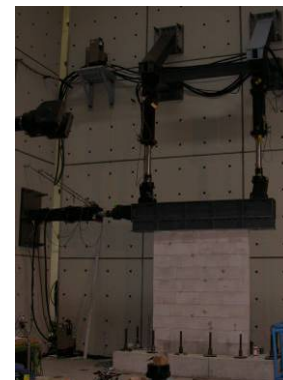
Figure 3: Complex test setup at EUCENTRE, Pavia, Italy: (a) scheme, (b) testing a masonry panel [2].
