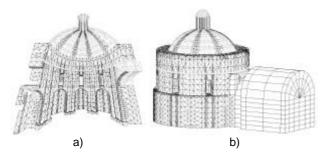
Figure 3: Numerical modeling of the church. (a) Halfmesh (inside view) and (b) total mesh (outside view)
