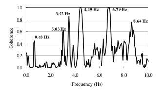
Figure 7: Coherence between records at points n4p3 (level 4) and n1p5 (level 1)
