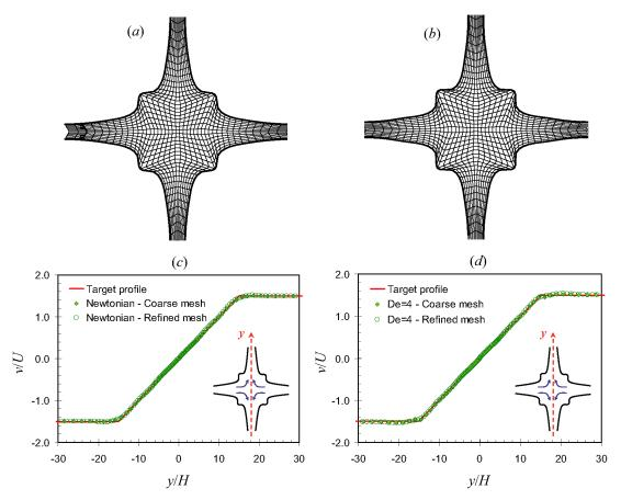
**FIGURE 2.** Optimized meshes calculated for (a) Newtonian fluid and (b) UCM fluid at De = 4. Velocity profiles along the vertical centerline (x = 0) for the optimized cross-slot flow geometries: (c) Newtonian fluid; (d) UCM fluid at De = 4.
