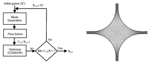
FIGURE 1. (a) Schematic illustration of the optimization cycle and (b) zoomed view of the coarse mesh used as initial estimate.
