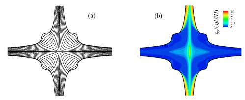
**FIGURE 3.** (a) Predicted streamlines and (b) contour plot of  $\tau_{yy}/(\eta U/H)$  for a UCM fluid at De = 4.
