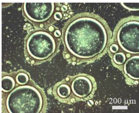
Figure 2.6. Optical microscopy images of microcapsules of orange flavour with whey protein/gum arabic coacervates, before drying (Weinbreck, 1977).
