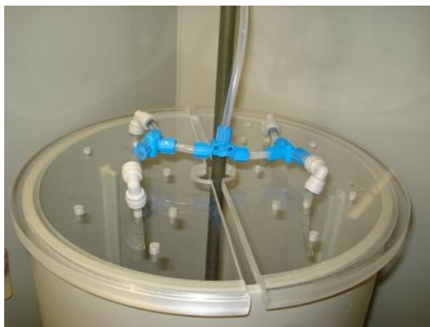
Figure 10 - Diffuser to add H 3 PO 4 .
