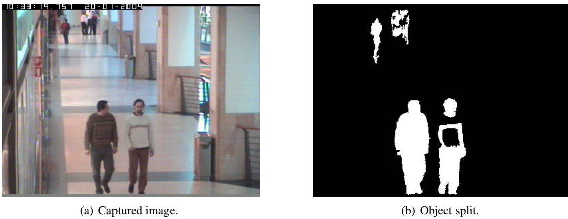
Figure 2.3: Example of an object split error where the segmentation represents a unique object as two distinct ones.
