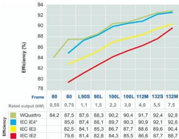
Figure 3 - Efficiency graph of the WEG WQuattro Hybrid motor compared to the IE standards
