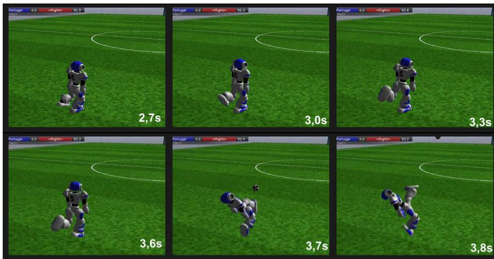
Figure 20. Sequence of the kick's poses placing and respective kick
