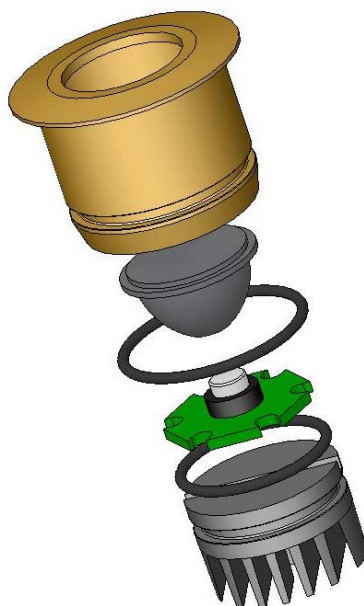
Figura 5.28 – Vista explodida foco Led 01
