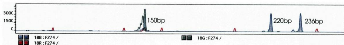
Figure 12: Pattern obtained after the separation of an amplification product of the D2S3010/D2S3016 duplex PCR in the automated genetic analyzer ABI PRISM® 310. In green (D2S3016): homozygote 150/150 bp; in blue (D2S3010): heterozygote 220/236 bp.
