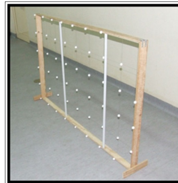
Figure V. Structure built for purposes of camera calibration.
