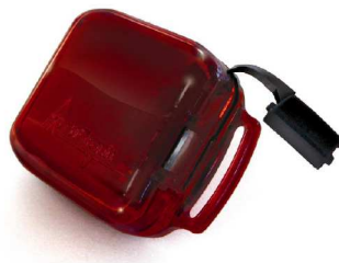
Figure 2. The uni-axial ActiGraph accelerometer (GT1M).
