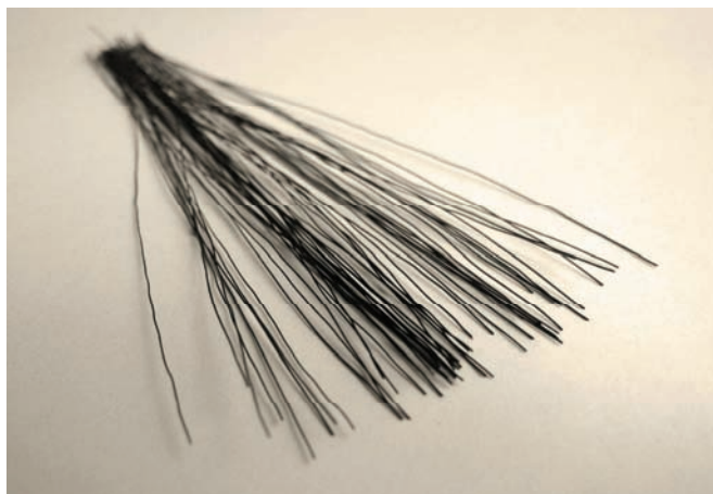
Figure 5.2 – Carbon molecular sieve hollow fibres from Carbon Membranes Ltd.
