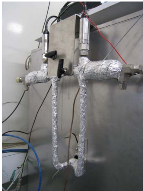
Figure A.5 – Heating tapes to avoid the reactants condensation.
