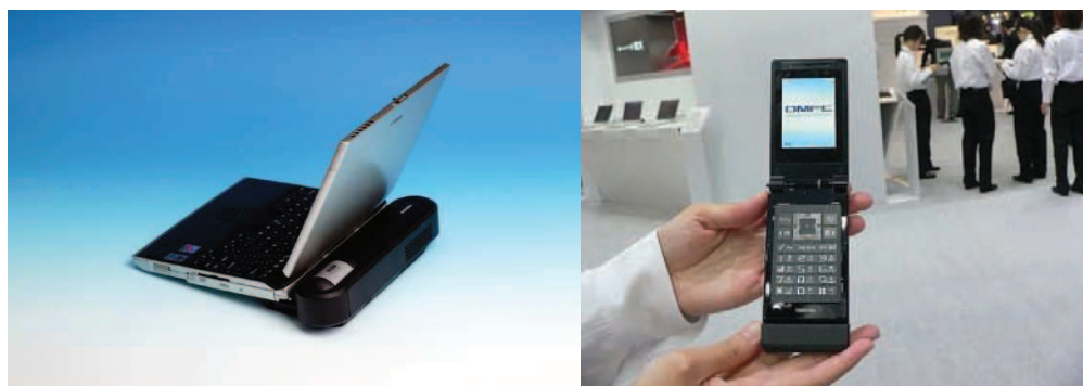
Figure 1.3 – Toshiba DMFC laptop prototype [18] (at the left); Toshiba DMFC cell phone prototype presented at CEATEC Japan 2008 conference [19] (at the right).
