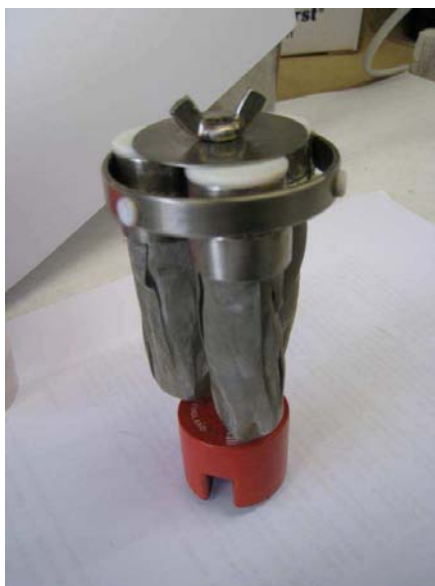
Figure A.4 – Gasket for holding the methanol steam reforming catalyst.
