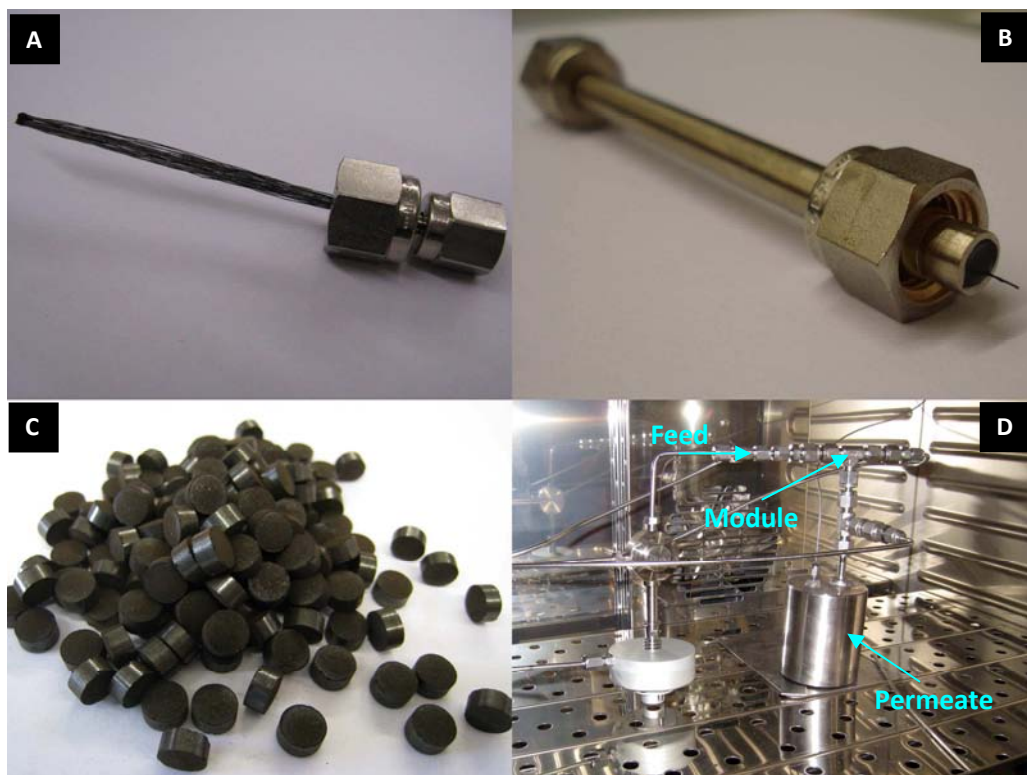
Figure A.8 – (A) – Membrane module with 15 fibers; (B) – Membrane module with 1 fiber; (C) – MSR catalyst; (D) – View of the membrane reactor module placed inside the oven.
