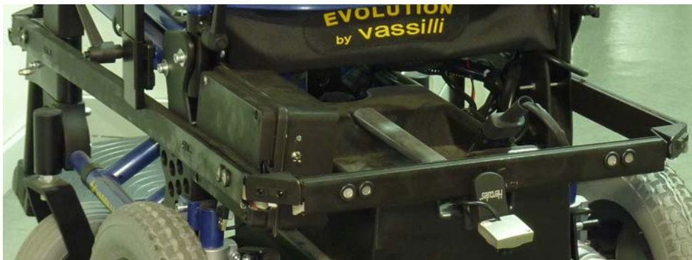
Figure 3.2: IntellWheels ' U-Shaped Sensor Bar with the Webcam also attached to it.
