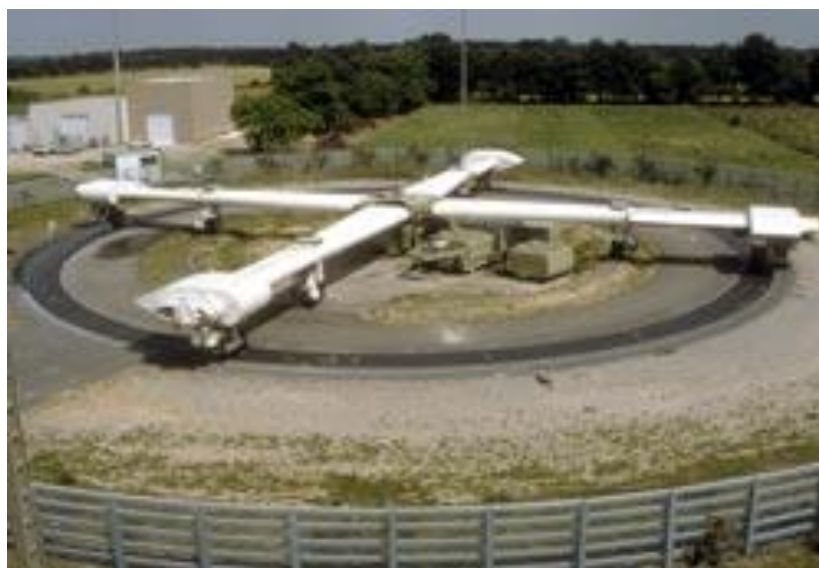
Figura 1-7 - Pavement Fatigue Carousel (Nantes)
