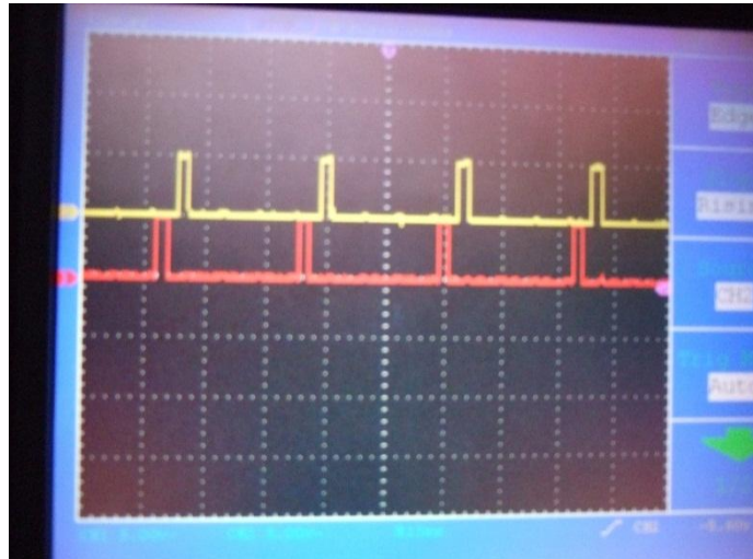
Figure 2.14 - Fuel Trigger (red) and Cam signal (yellow)
