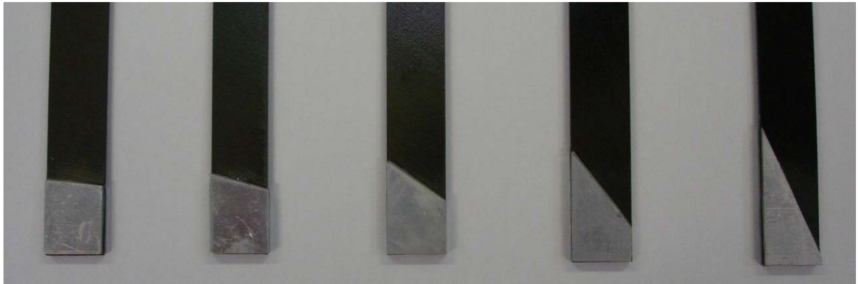
Figure 6: Geometry of the tabs used in this study for each fiber orientation respectively
