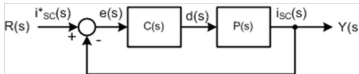
Figure 5.7: Closed loop current control Block Diagram
