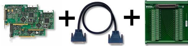
Figure 3.7: Voltage Measurement Hardware
