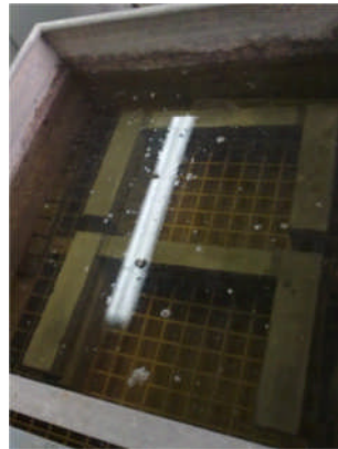
Figure 3.21 – Curing of Concrete
