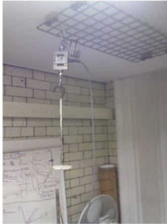
Figure 3.33 – Load Cell Calibration
