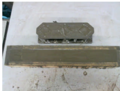
Figure 3.28 – Beam after Casting
