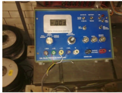
Figure 3.40 – Strain Indicator Registering Strain Values from Load Cell
