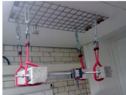
Figure 3.38 – Load Cell Placed in the Middle of the Bar
