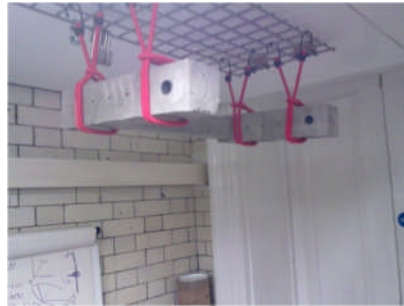
Figure 3.35 – Simulation of the Free Support
