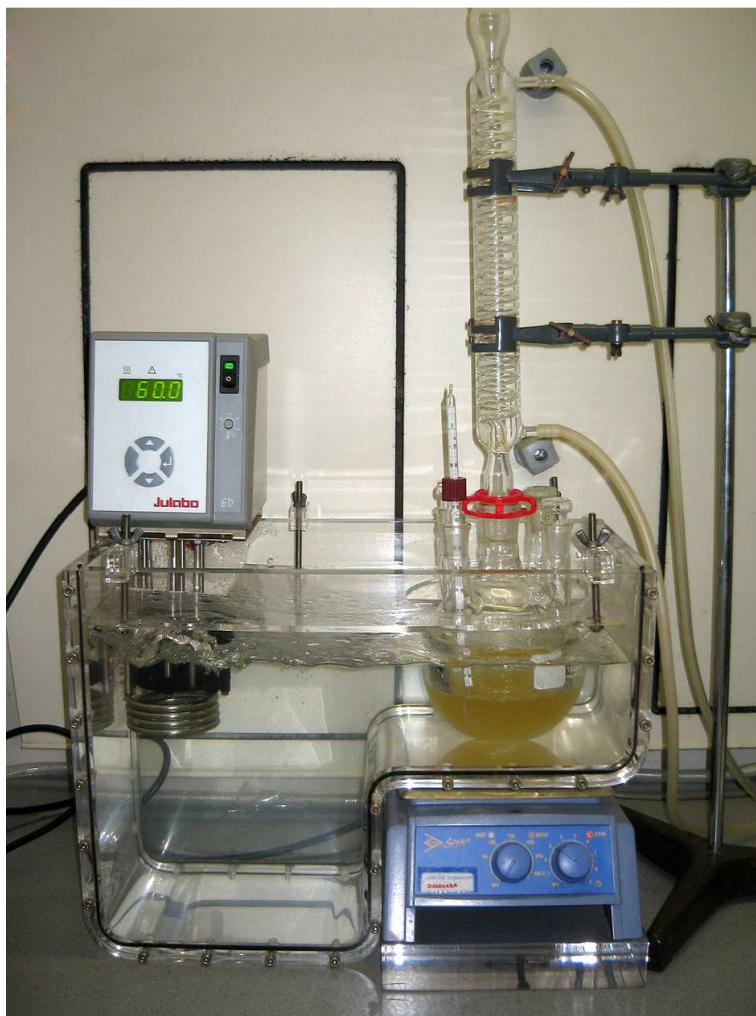
Figure 2.3. Reactor used for homogeneous synthesis and designed acrylic bath.
