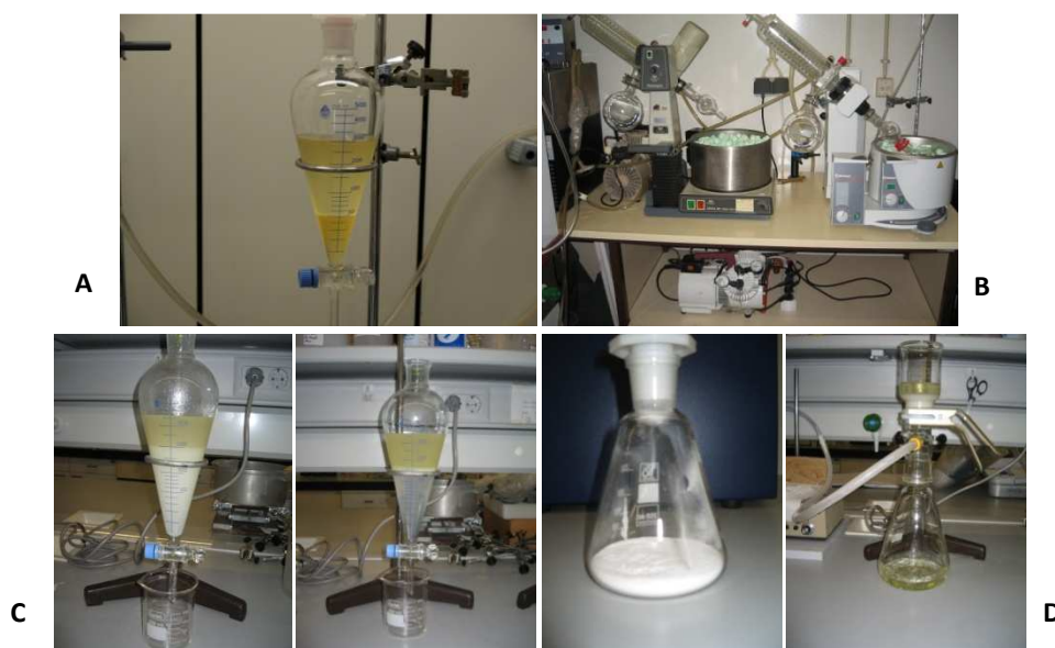
Figure 2.4. Separation and purification of biodiesel: A. phase separation; B. methanol recovery; C. washing; and D. drying.
