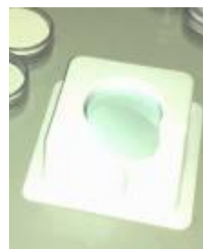
Filtro SKC de PVC 37mm 5,0 µm
