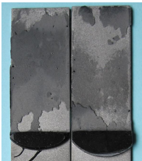
Figure 21- Fracture surface of a joint without fibers (first trial).
