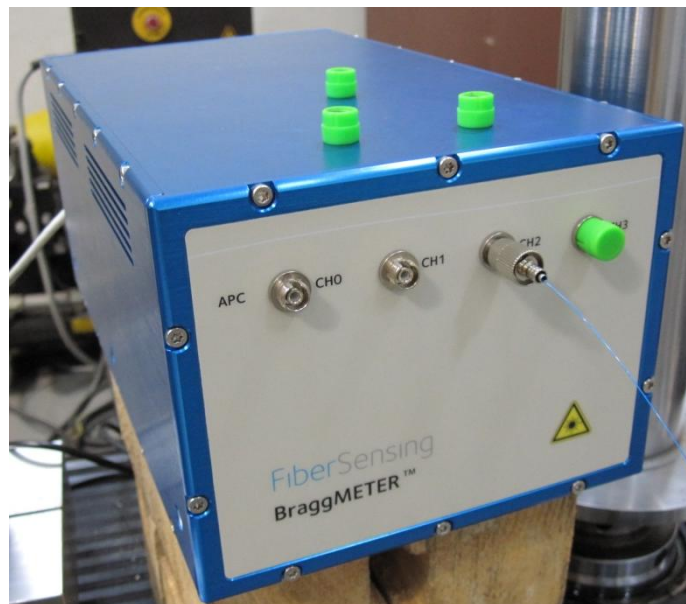
Figure 61- BraggMETER FS2100 | FS2200 measurement unit.
