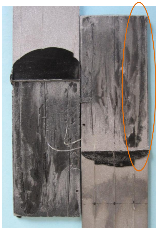
Figure 30- Fracture surface of a joint (third trial).
