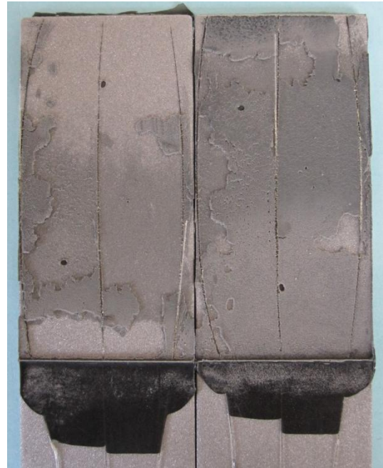
Figure 35- Fracture surface of another joint (fourth trial).
