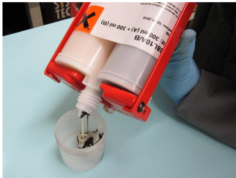
Figure 44- Adhesive's extraction using an adhesive applicator gun.
