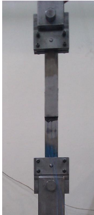
Figure 64- Adhesive joint assembled to MTS machine.
