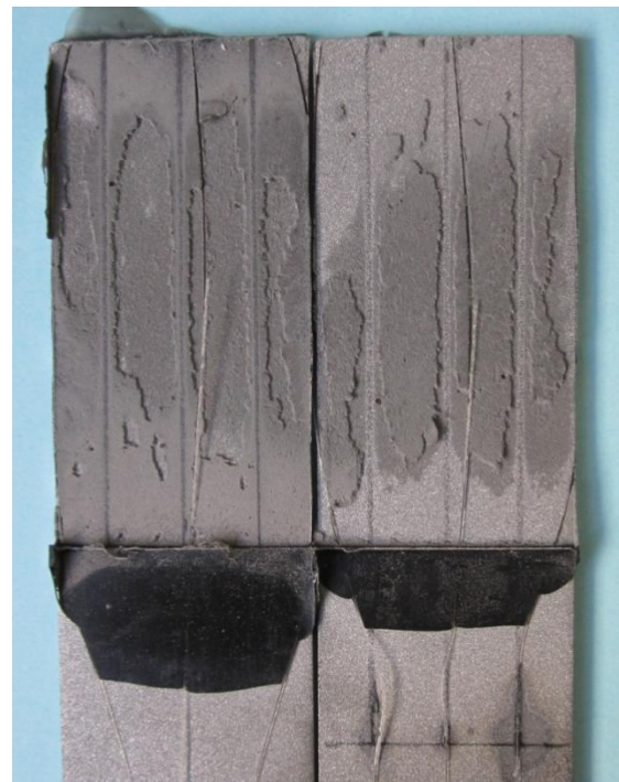
Figure 26- Fracture surface of a joint with fibers (second trial).
