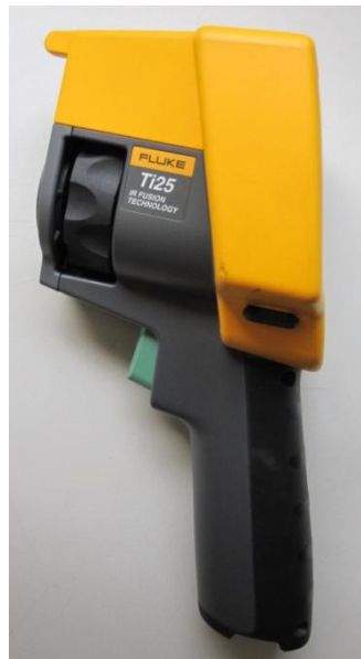
Figure 42- FLUKE Ti25 infrared camera.
