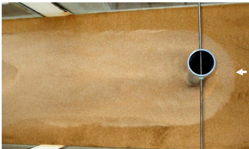
Figura xxiv - Final erosion cavity, top view (test B2).
