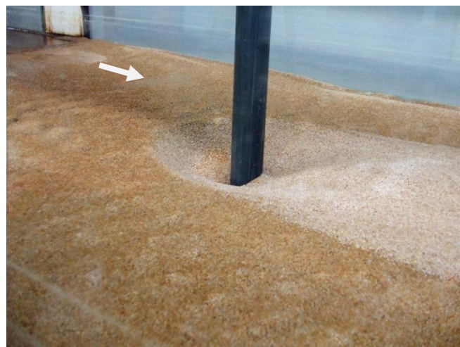
Figura xvii - Detail of the erosion cavity near the pier (side view, test A4).
