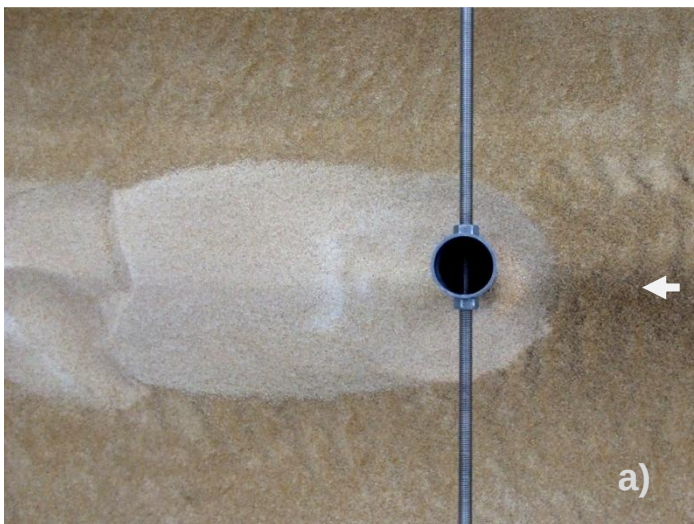
Figura xviii- Final erosion cavity of test A4. a) Top view. b) Downstream view.
