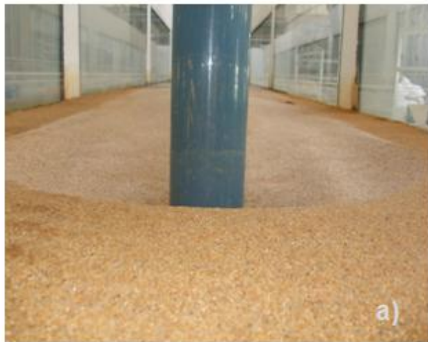
Figura xxiii - Final erosion cavity. a) Upstream view. b) Top/upstream view.
