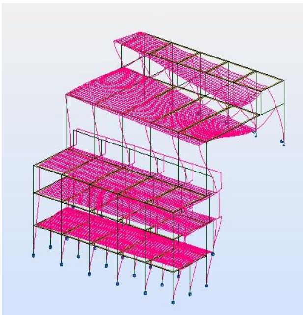
Fig.5.14 – Modo 6 (freq. 4.49 Hz)
