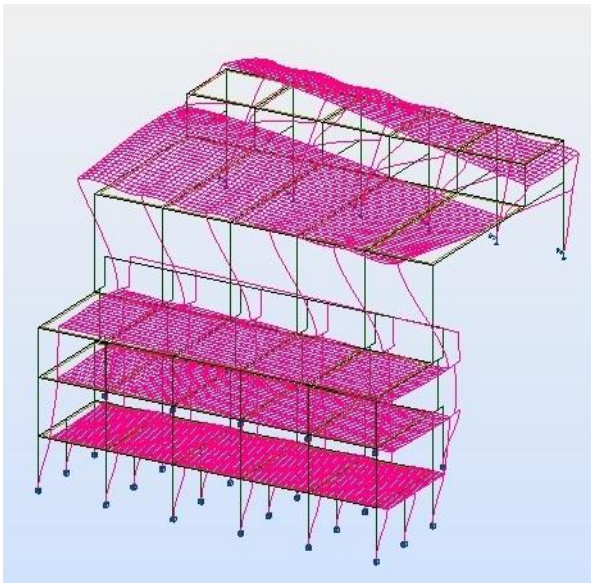
Fig.5.12 – Modo 4 (freq. 3.55 Hz)
