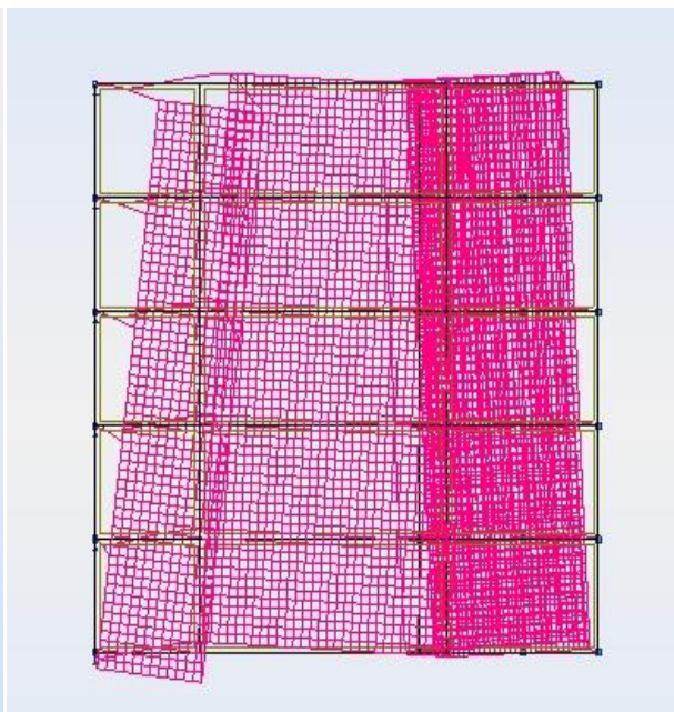
Fig.5.14 – Modo 6 (freq. 4.49 Hz)
