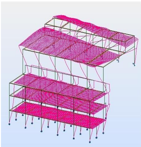
Fig.5.13 – Modo 5 (freq. 3.90 Hz)
