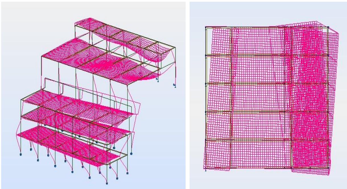
Fig.5.21 – Modo 13 (freq. 6.3 Hz)
