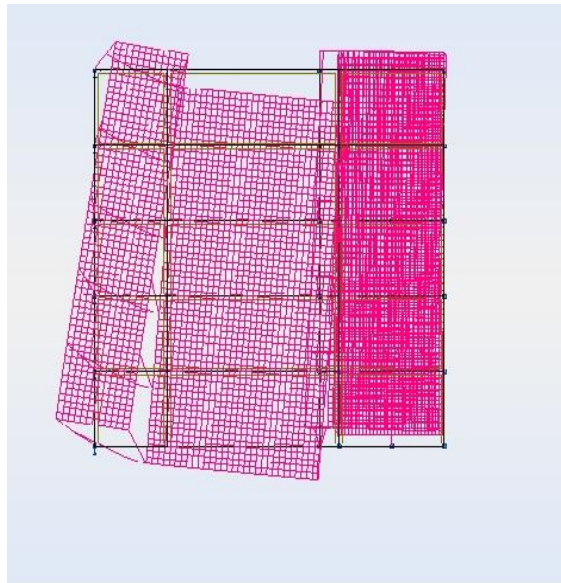
Fig.5.12 – Modo 4 (freq. 3.55 Hz)
