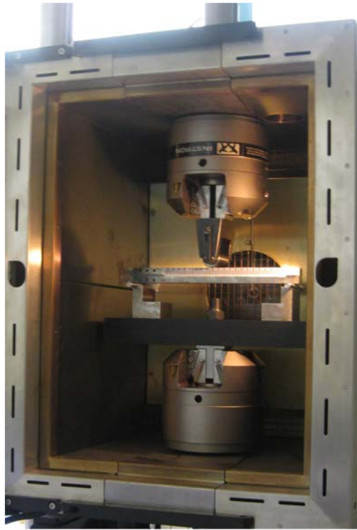
Fig. 5 – ENF specimens set-up.
