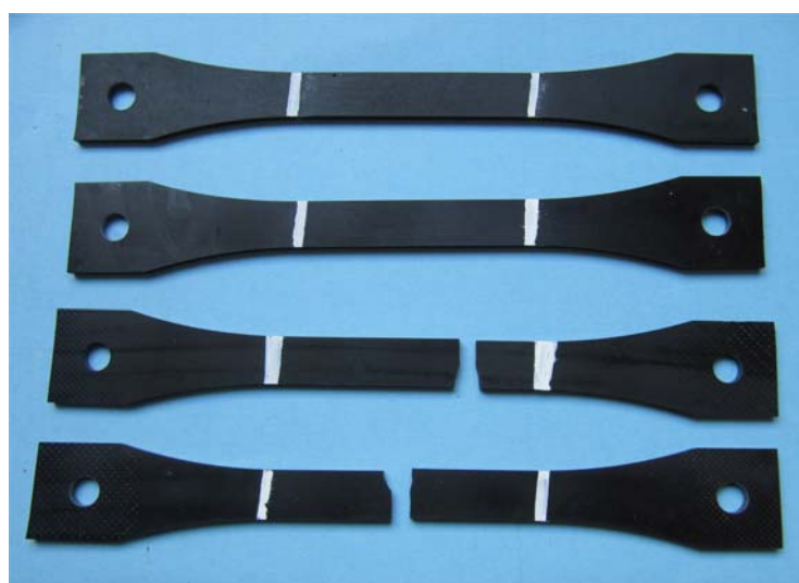
Fig. 4 – Bulk specimens before and after tests.
