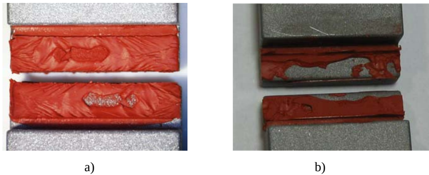
Fig. 6 Failure mode in TAST specimens: a) AS1805 RTV adhesive; b) RTV106 adhesive.
