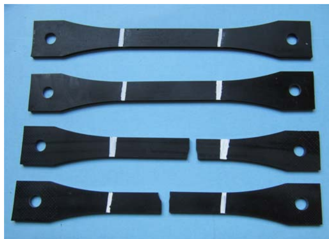
Fig. 4 – Bulk specimens before and after tests.
