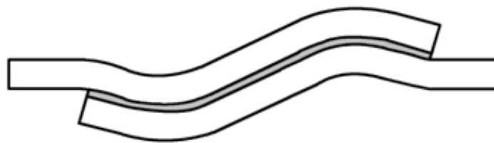
Figure 5. “Wavy” lap joint configuration (redrawn from [18]).
