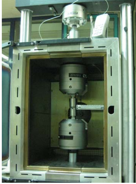
Fig. 8 – DCB specimens set-up.
