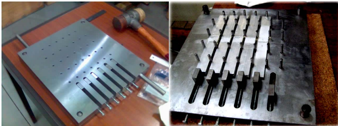
Fig. 4 Mould for SLJ specimens fabrication.
