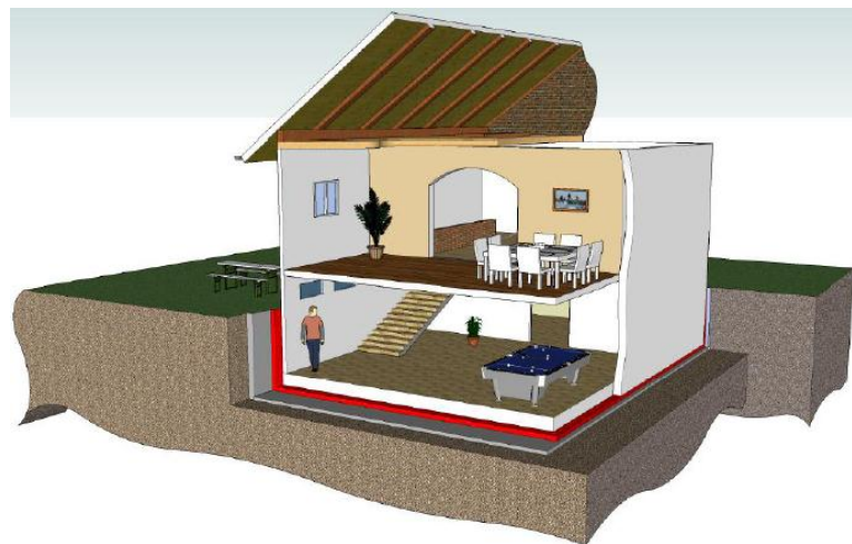
Fig. 18 – Building elastically supported [10]
