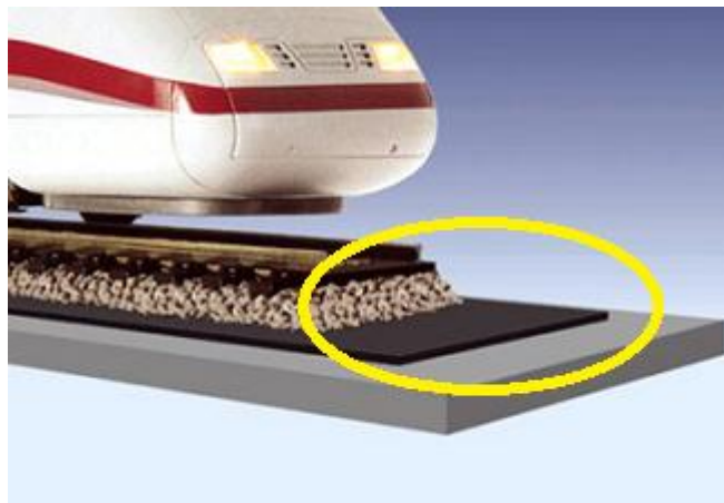
Fig. 15 – Ballast mat application
