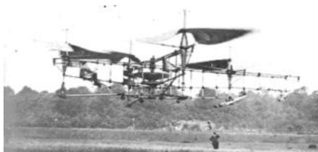
Figura 2.2 - Quadrotor Etienne Oemichen, 1922 [3]
