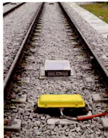
Figura 13 – ATP (Automatic Train protection)
