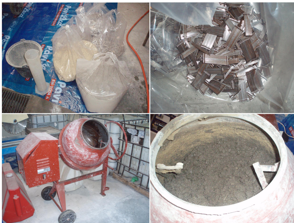
Fig. 4.13: Making fibre-reinforced concrete
