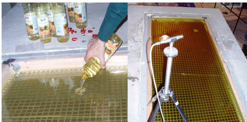
Fig. 4.21: Filling the test sample (left) and then testing the vegetable oil (right)
