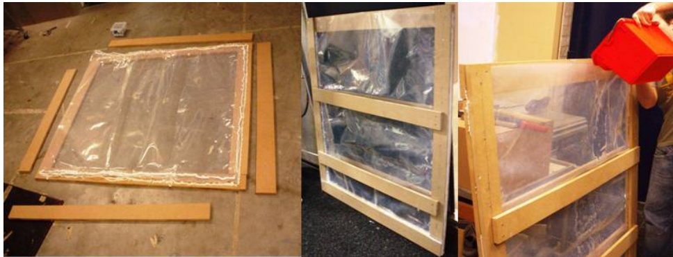
Fig. 4.9: Initial test sample: building the sample (left) and then filling it with water (right)
