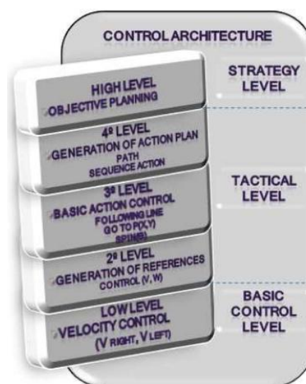
Figure 2.3 - Intellwheels Control Architecture from [2].
