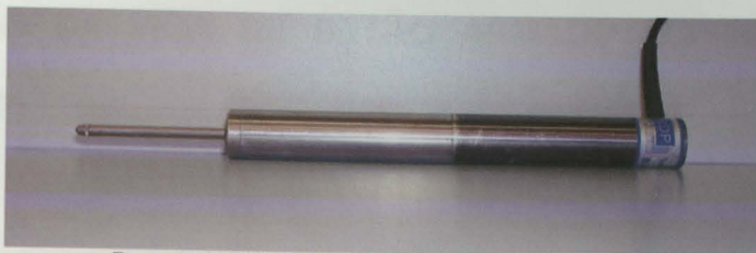
Figura 9 – LVDT's ( Linear Variable Differencial Transformer )
