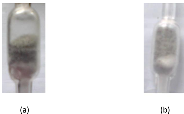
Figure 3.4.2.1 – Images of the reactor half filled (a) and totally filled (b).
