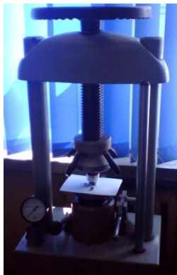
Figure 3.4.1.1 – Hydraulic press used to prepare the tablets.
