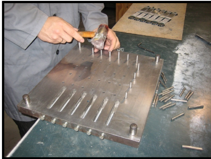
Figure F 14 –Mould pin replacement.
