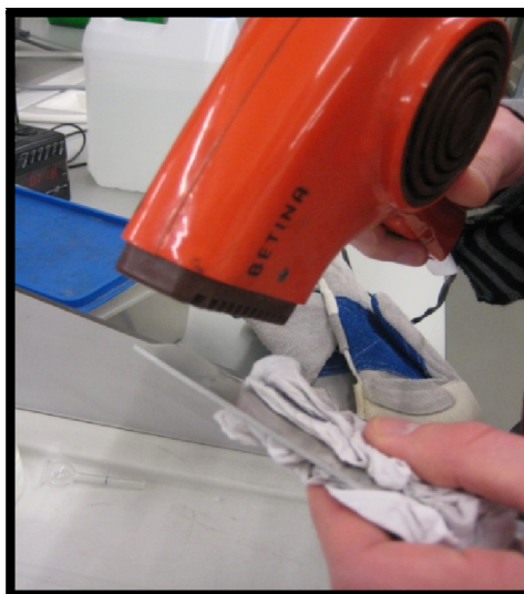
Figure G 10 – Adherends drying.
