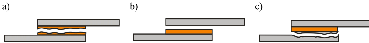
Figure 61 - Different types of adhesive joint failure; a) cohesive failure b) adhesive failure c) adherend failure.
