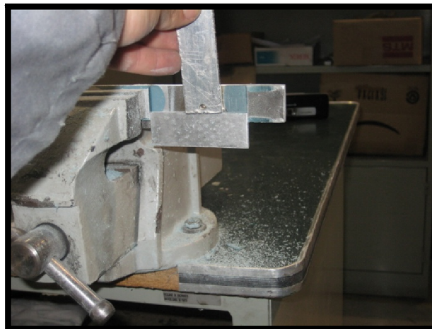
Figure F 18 – Spacers removal.
