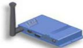
Figura 10.3 - Mesh Gate (MG) [41]
