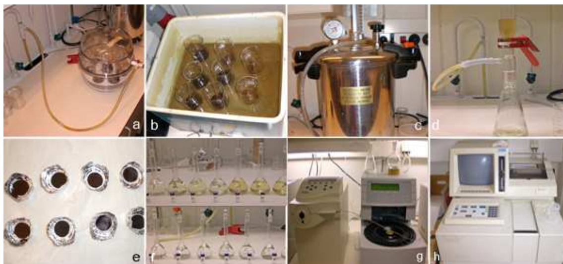
Figure 3.7 – Lignin and carbohydrate analysis steps: a) evacuation of the beakers; b) beakers placed in a 30°C water bath; c) autoclave; d) filtration of the content of a beaker; e) Klason lignin after filtration; f) concentrated and diluted solutions after filtration; g) HPLC; h) spectrophotometer used to measure the absorbance of the diluted solutions in order to calculate the acid soluble lignin content.
