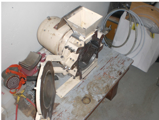
Figure 3.2 – Wiley mill used for grinding both Scots pine heartwood and Blue gum.
