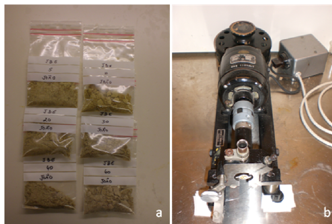
Figure 3.6 – a) wood residue samples; b) grinder used to grind the wood residue samples.
