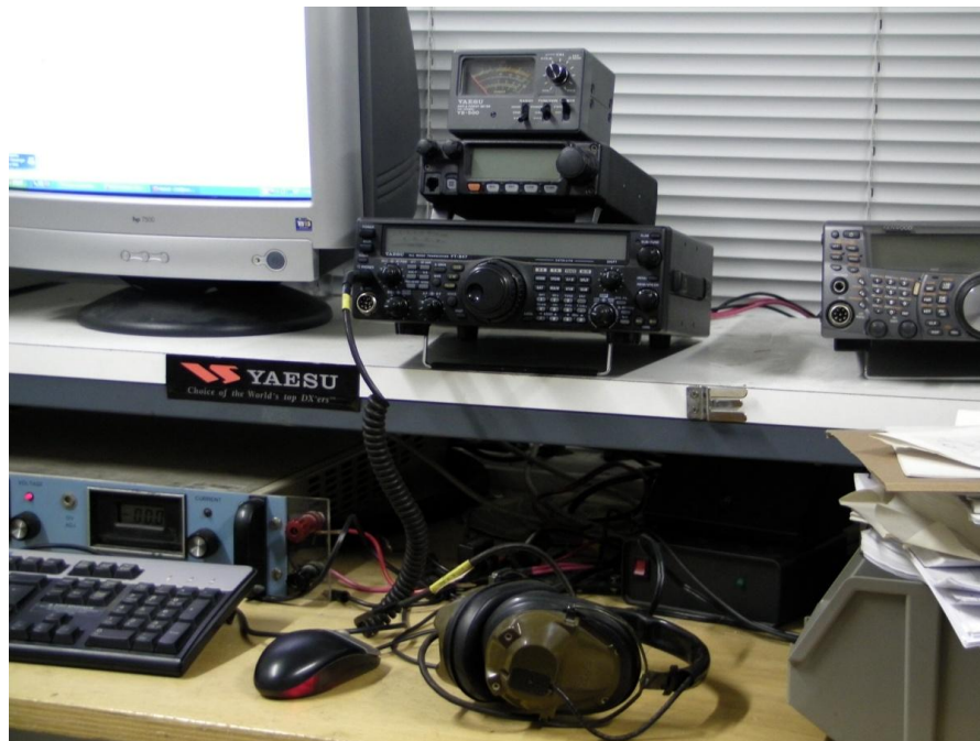
Figure 3.3 - Receiver and computer used to record the Argos signals in the ground station.
