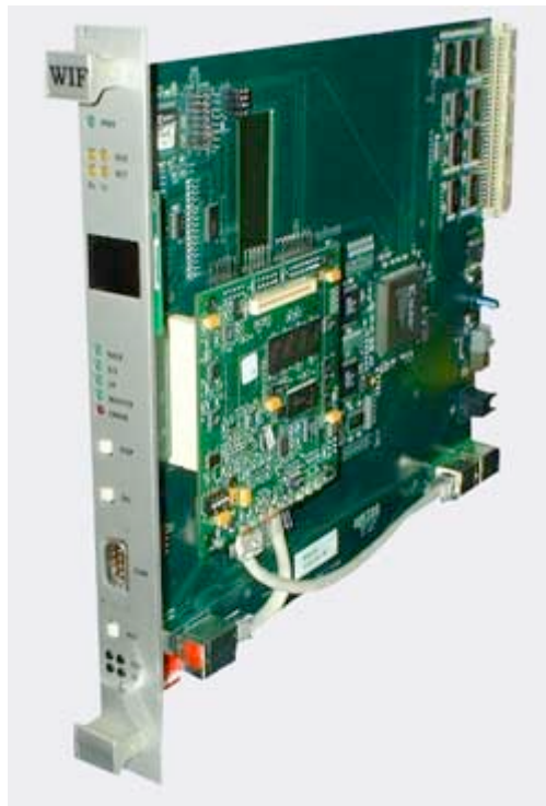
Figura 4.3: Placa WIF - Workstation Interface card
