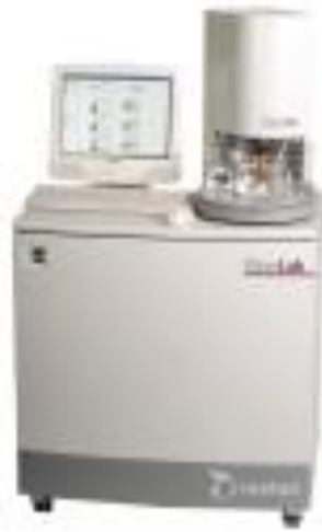
Figure 22 -kajaaniFiberLab equal to the used one (Metso Automation, 2010)).
