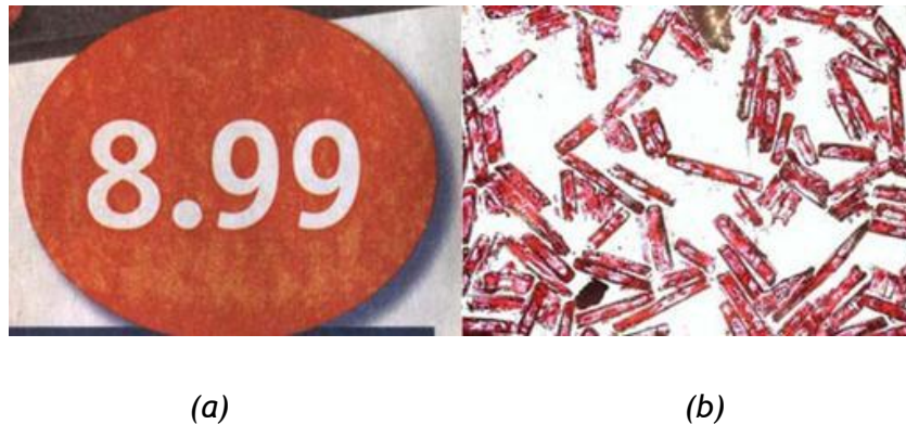
Figure 4 - a) Shows printing defects, on the red area, caused by linting. b) Magnification of lint deposits where is possible to see red inked ray cells (Courtesy of SCA).
