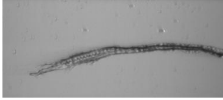
Figure 25 - Normal fiber image from kajaaniFiberLab cross-section camera.
