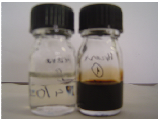
Figure 72 - Final solutions from Methylcellobiose hydrolysis at 80°C in \text{LiCl}\cdot 4\text{H}_2\text{O} and in \text{ZnCl}_2\cdot 4\text{H}_2\text{O} .
