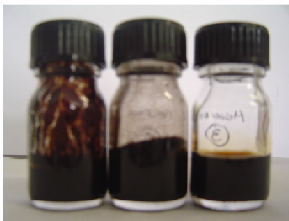
Figure 55 - Final solutions from Glucose stability in \text{ZnCl}_2 \cdot 4\text{H}_2\text{O} at 100^\circ\text{C} and 30 bar \text{N}_2 .
