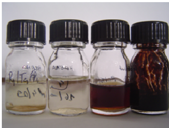
Figure 23 - Final solutions from Cellobiose hydrolysis at 100^\circ\text{C} , 30 bar \text{N}_2 and after 60 minutes, in: \text{H}_2\text{O} , 1% \text{ZnCl}_2 , \text{ZnCl}_2 \cdot 4\text{H}_2\text{O} , and \text{ZnCl}_2 \cdot 2\text{H}_2\text{O} .
