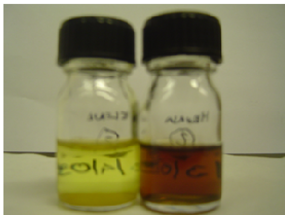
Figure 74 - End solutions from Methylcellobiose hydrolysis at 100°C in \text{LiCl}\cdot 4\text{H}_2\text{O} and in \text{ZnCl}_2\cdot 4\text{H}_2\text{O} .
