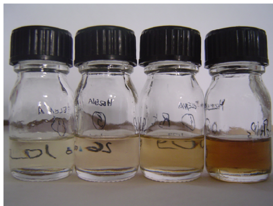
Figure 25 - Final solutions from Methylcellobiose hydrolysis in \text{ZnCl}_2 \cdot 4\text{H}_2\text{O} at 80^\circ\text{C} after 30, 90, 120, and 240 minutes of reaction.
