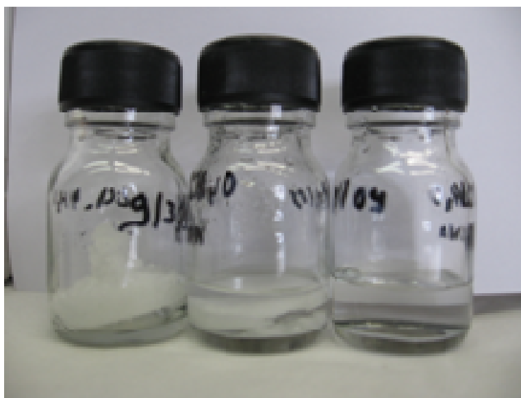
Figure 14 - Bottles with different concentrations of lithium chloride ( \text{LiCl} ): \text{LiCl} \cdot 1\text{H}_2\text{O} (10g), \text{LiCl} \cdot 2\text{H}_2\text{O} (10g) and \text{LiCl} \cdot 4\text{H}_2\text{O} (10g).
