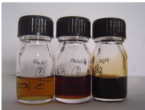
Figure 17 – Final solutions from Cellobiose hydrolysis in ZnCl_2 \cdot 4H_2O at 100°C after 30, 60, and 120 minutes.
