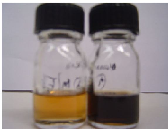
Figure 71 - Final solutions from Cellobiose hydrolysis at 80°C in LiCl·4H 2 O and in ZnCl 2 ·4H 2 O.
