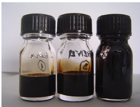
Figure 18 - Final solutions from Cellobiose hydrolysis in \text{ZnCl}_2 \cdot 4\text{H}_2\text{O} at 130^\circ\text{C} after 10, 30, and 60 minutes.
