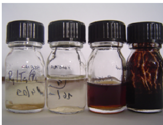
Figure 59 - Final solutions from Cellobiose hydrolysis at 100^\circ\text{C} in \text{H}_2\text{O} , 1% \text{ZnCl}_2 , \text{ZnCl}_2 \cdot 4\text{H}_2\text{O} and \text{ZnCl}_2 \cdot 2\text{H}_2\text{O} .
