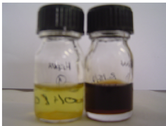
Figure 73 – Final solutions from Cellobiose hydrolysis at 100°C in \text{LiCl}\cdot 4\text{H}_2\text{O} and in \text{ZnCl}_2\cdot 4\text{H}_2\text{O} .
