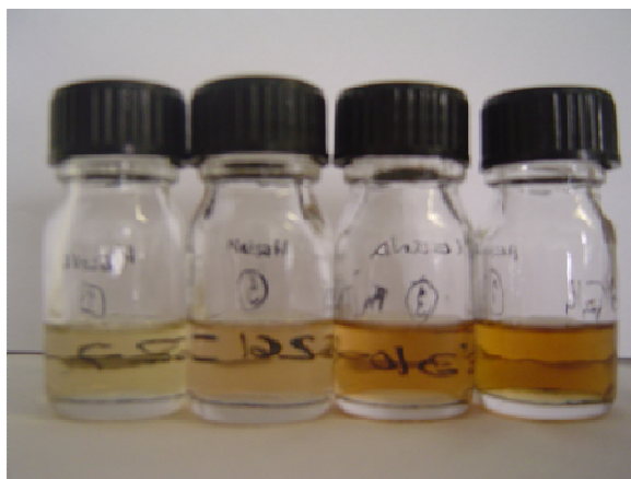
Figure 16 - Final solutions from Cellobiose hydrolysis in ZnCl_2 \cdot 4H_2O at 80°C after 30, 90, 120, and 240 minutes of reaction.
