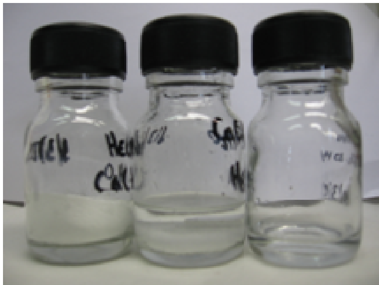
Figure 15 - Bottles with different concentrations of calcium chloride ( \text{CaCl}_2 ) : \text{CaCl}_2 \cdot 1\text{H}_2\text{O} (10g), \text{CaCl}_2 \cdot 4\text{H}_2\text{O} (10g) and \text{CaCl}_2 \cdot 20\text{H}_2\text{O} (10g).
