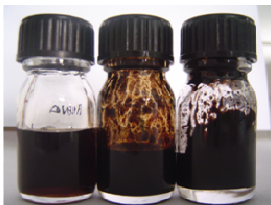
Figure 27 - Final solutions from Methylcellobiose hydrolysis in \text{ZnCl}_2 \cdot 4\text{H}_2\text{O} at 130^\circ\text{C} after 10, 30, and 60 minutes of reaction.
