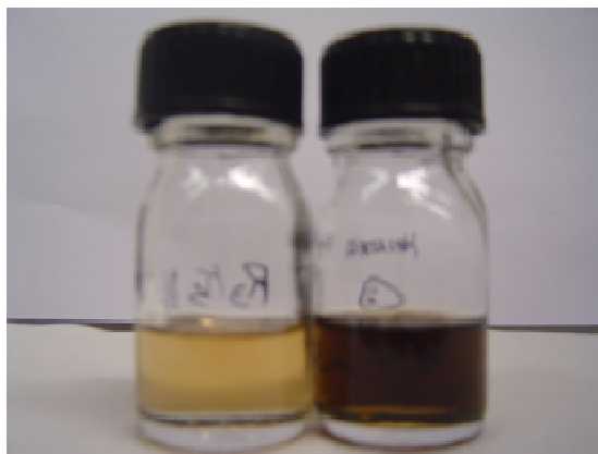
Figure 31 – Final solutions from Methylcellobiose hydrolysis in \text{ZnCl}_2 \cdot 4\text{H}_2\text{O} at 80^\circ\text{C} during 120 minutes without and with HCl.
