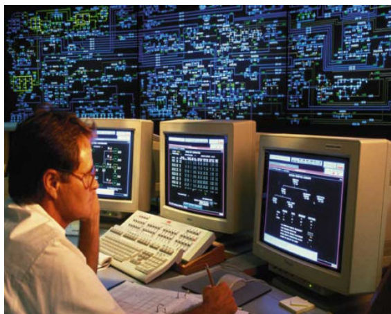
Figure 1.1: Central station of a SCADA system.
